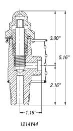
Sherwood's 1214 Series is designed for use in applications using chlorine gas, chlorine liquids, corrosive gases, insecticides & fumigants, preservatives and bleaching agents.
